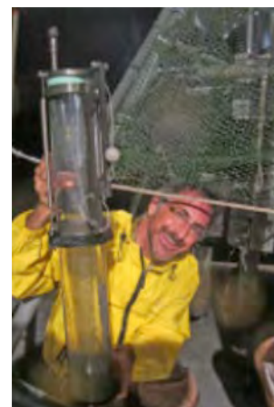
After recovering sediment cores from the Gulf, Hastings removes the sediment core from the sampler. Frequently, the cores are extruded on board the ship. (Photo credit: David Hastings, Eckerd College)
