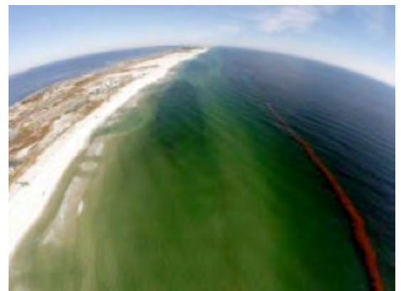
This aerial photo, taken from the camera-equipped drone, shows a mile-long dye strip injected outside the surf zone.
