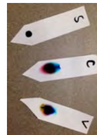
Results from an ink chromatography experiment using three different black markers.
