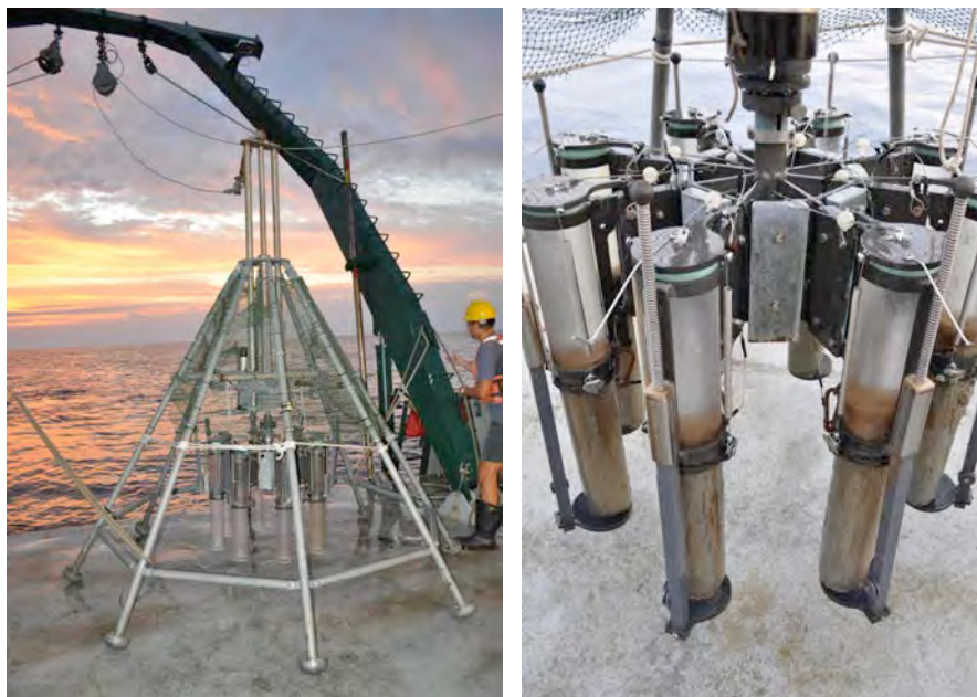
Multi-corer on deck and an up close view of full cores. (Photo credit: Amy Baco-Taylor, FSU)
