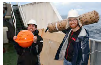
Johannes Rohrs and Kai Christensen prepare to deploy two types of surface drifters. The drifter in the cardboard box unfolds once in contact with water. (Photo by: Göran Broström)
