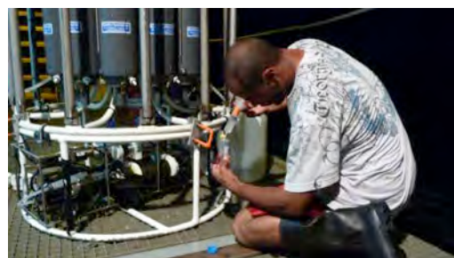
FSU PhD student Nick Myers collects water samples from the CTD (connectivity, temperature, depth) during a research cruise to analyze for the presence of methane ( \text{CH}_4 ).
