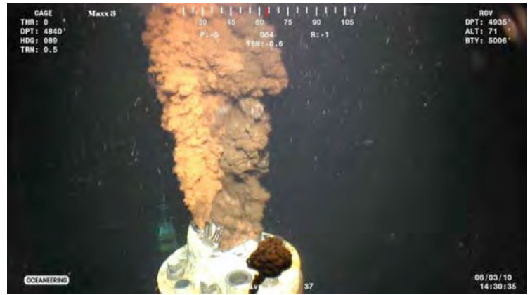
The Macondo well was two days from completion when high-pressure methane gas from the well expanded into the riser, and rose into the drilling rig, where it ignited into an explosion. Experts estimated that oil flowed from the well at a rate of 62,000 barrels per day.
