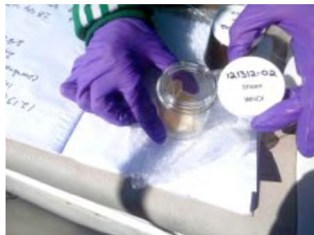
After researchers retrieved oil-coated screens used to collect samples from surface sheens, each screen was sectioned into several pieces for analyses. Some were reserved for DNA extraction; others analyzed for drilling fluids and shared with the National Oceanic Atmospheric Administration for standard petrochemical analyses. (Photo by Christoph Aeppli, WHOI)
