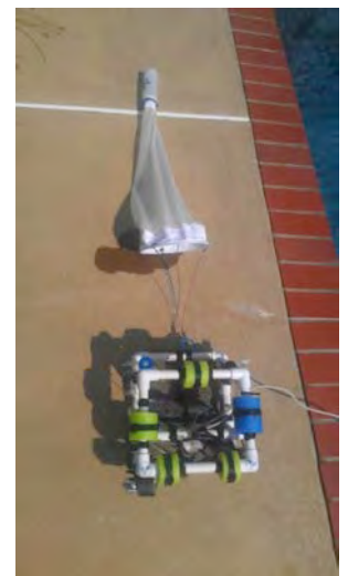
ROV with a plankton tow made by Deep-C intern Rachel Holliday.
